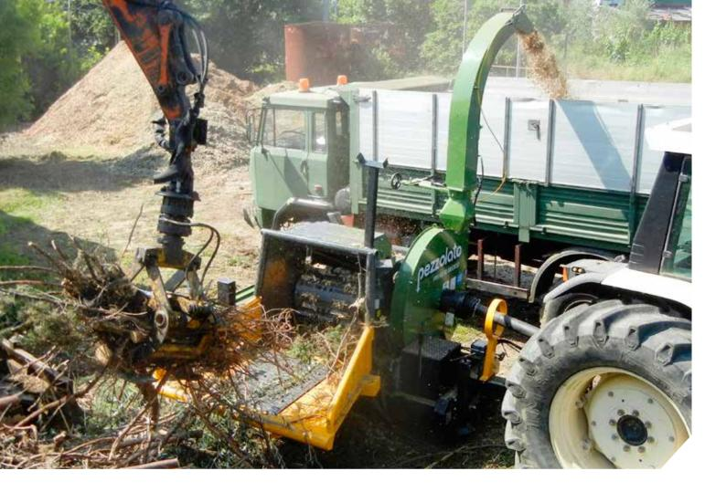
using the machine. A large horizontal roller with pawls supported by a belt placed in the inner part of the hopper allow to insert the material easily.
