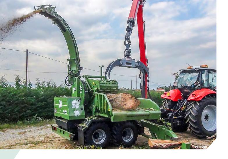
work at a low speed (less than 600 revs) to help reduce dust and increase wood chip quality. Each standard installation includes a single axis trailer which provides compactness and increases agility and manoeuvrability in tight spaces. With its cutting system that is interchangeable where required, the drum makes these chippers ideal for the production of wood chips used with domestic boilers, large power plants or gasifiers.
