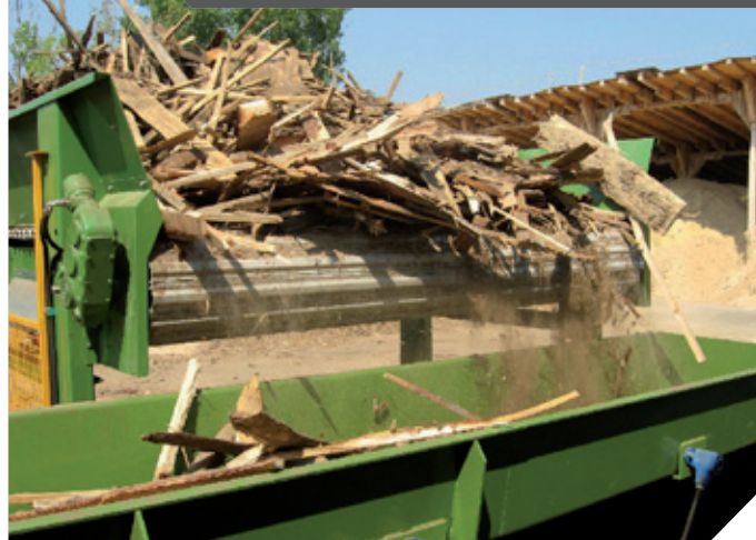
Loading table with closed chains
